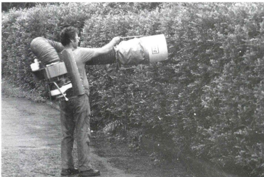
Figure 4 - D-VAC machine aspirating D. citri on ornamental Murraya paniculata hedges Tampon 600 m, Réunion
