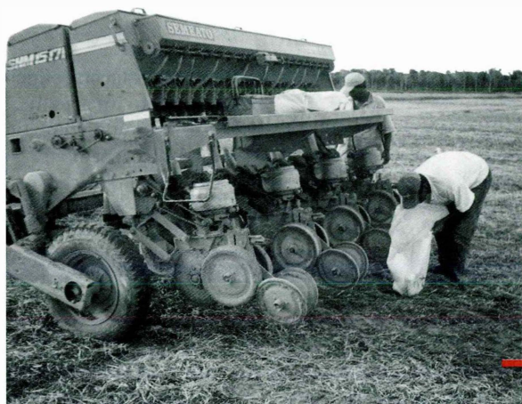
Mechanized direct sowing of maize into soybean residues.
