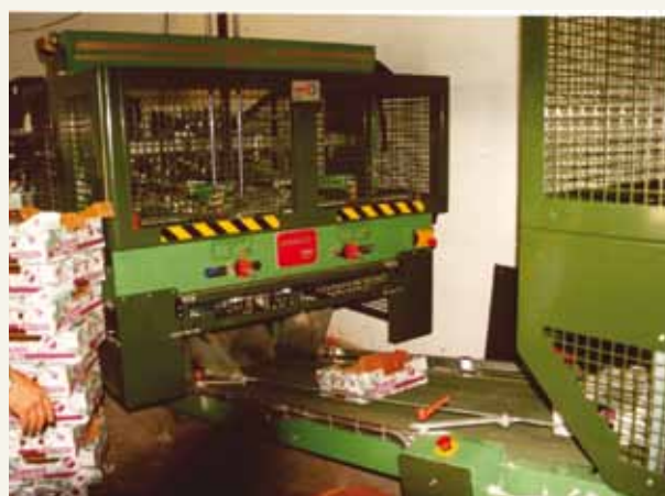
Box gluing machine (Brazil). Various African stations use this material instead of manually assembled boxes (saving cardboard, increased strength, etc.) (Photo - Jean-Yves Rey)
