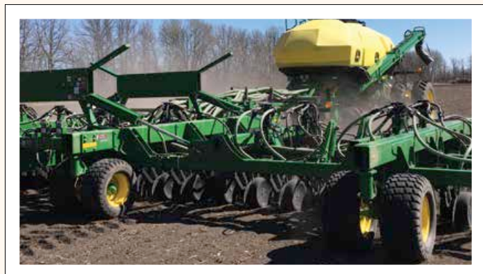
Figure 4.15. Air disk drill. Source: Kristen MacMillan, University of Manitoba.
