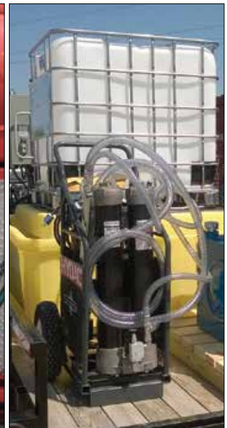
OFS Filtration Station with HPU.
