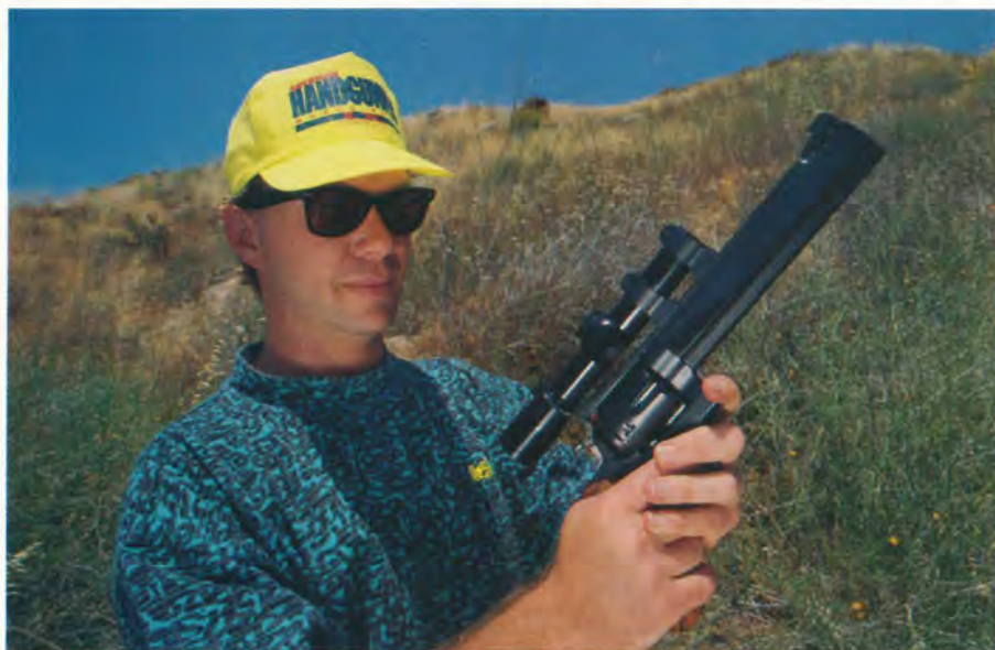
The Miller MercComp incorporates a mercury filled underlug and a dual port compensator. The system is astonishingly effective at dampening felt recoil. Note the tasteful installation of the handmade front sight in a precise dovetail cut. We test fired the Miller Redhawk (right) at a southern California range with AH reader Scott Sturm.
