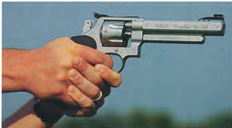
A John Nowlin custom .45 ACP pingun features a slab sided Shilen match barrel, Metaloy finish and an incredibly smooth DA trigger.
