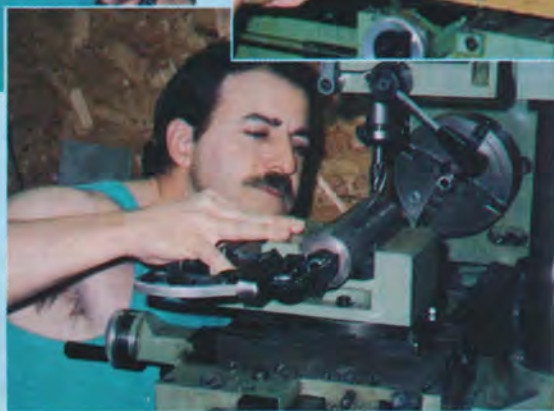
Kent Miller holding up the 2.5" Krieger barrel blank that became the slab sided beauty it is now after Kent went to work making steel chips. The pile is everything that didn't look like a barrel!
