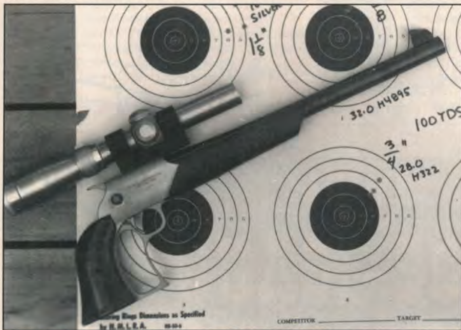
The M.O.A. single-shot pistol is capable of sub-MOA (hence the name) at 100 yards. John's test gun is chambered in .250 Savage, a good hunting round.
