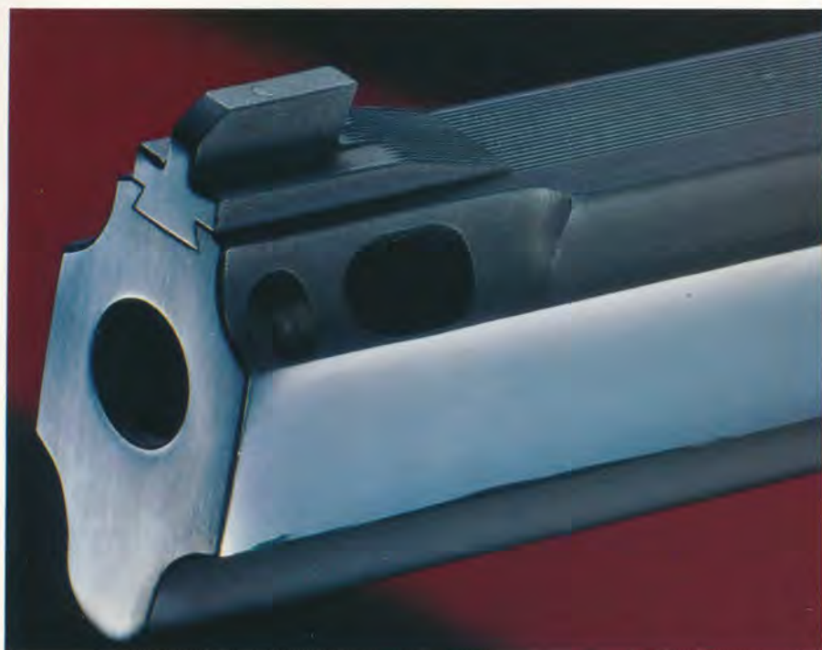
The Miller MercComp incorporates a mercury filled underlug and a dual port compensator. The system is astonishingly effective at dampening felt recoil. Note the tasteful installation of the handmade front sight in a precise dovetail cut. We test fired the Miller Redhawk (right) at a southern California range with AH reader Scott Sturm.
