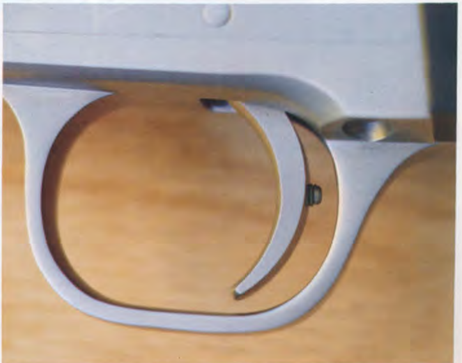
The trigger includes an over-travel stop, a nice custom touch on a factory gun.
