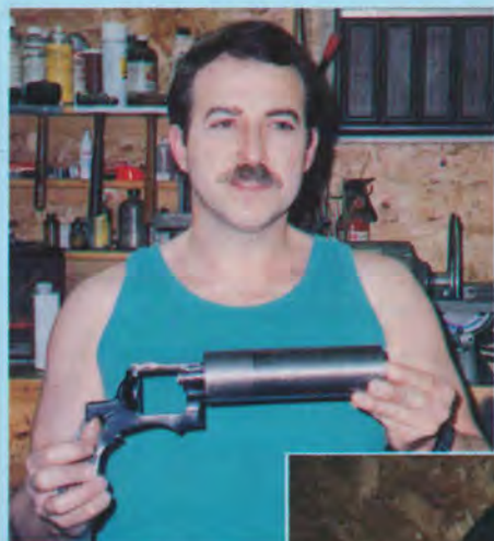
Kent Miller holding up the 2.5" Krieger barrel blank that became the slab sided beauty it is now after Kent went to work making steel chips. The pile is everything that didn't look like a barrel!
