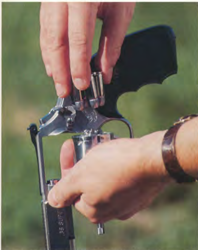
An unusual conversion of a S&W Model 27 to .38 Super. Since full-moon clips are fast to load, pin shooters prefer them to speed loaders, thus the impetus for this conversion.
