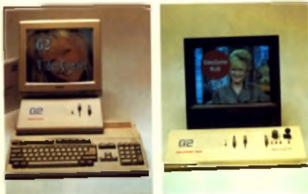
Top Left: The Videocentre is the same as the VC Plus, but without the wipe controls. Top Right: Some spectacular titling effects are possible using the wipe function.
