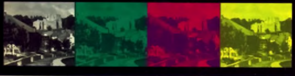
Four colour printing involves each image being broken down into cyan, magenta, yellow and black components.
