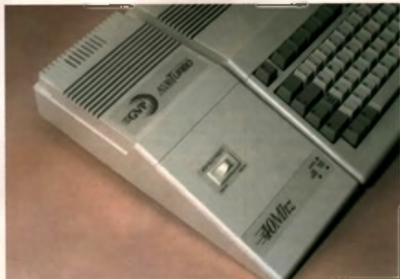
The GVP A530 Turbo may look like just another hard disk interface, but the beige exterior conceals the power to turn an A500 into a high-powered workstation.
