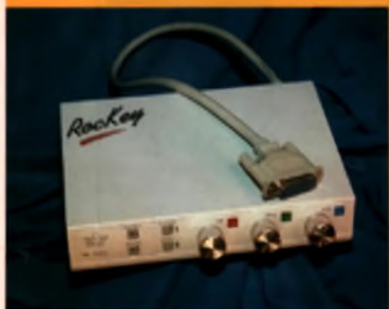
The Rockey unit is the world's most affordable colour separation overlay system (but you do need a genlock as well)
