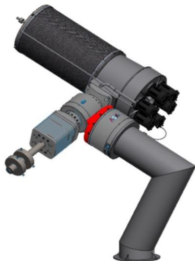
Fig. 2 The DREAMS telescope consists of a 0.5m optical telescope assembly that feeds a six-channel infrared camera payload [8]
