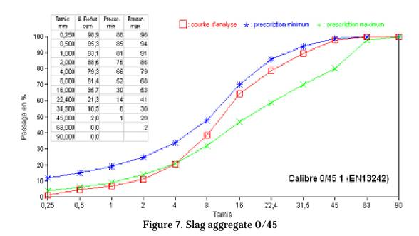
In Figure 7. we can see red line, property of slag product 0-45; and minimum and maximum requirement of EN 13242,
