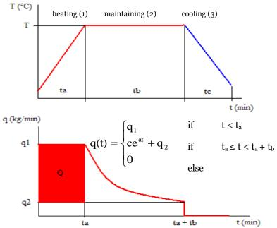
Figure 3. Development of temperature and steam mass flow in function of time Product-dependent data calculated from the sterilization curves:
