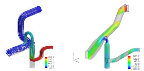
Figure 5. Simulation CFD – whole ductwork
