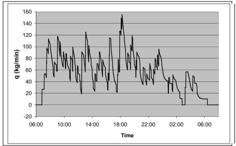
Figure 4. Total steam requirements of multiple autoclaves operating simultaneously
