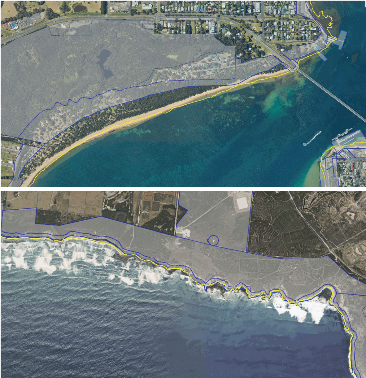
Figure 4.4 Examples of variations in alignment of Crown land along the coast where the boundary is ambulatory and defined by high or low water mark. All Crown land is shaded and the coastline is shown in yellow. Coastal reserve Crown land parcels are outlined in blue. Top: Phillip Island Coastal Reserve. Bottom: Narrawong Coastal Reserve.
