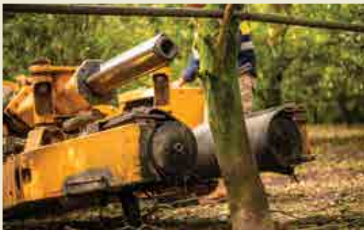
Tree shakers must be well maintained so the pads and heads are in good order with the right grip strength to suit the variety and girth of the tree.
