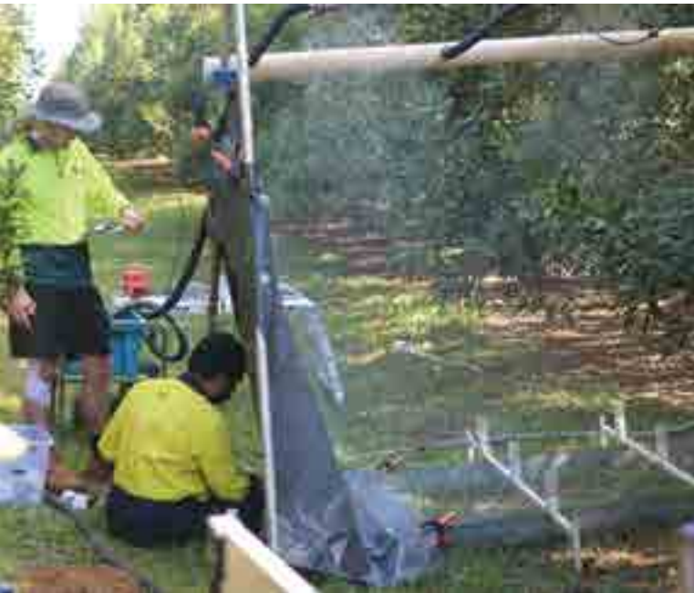
Luke Griffin and Sushil Pandey from DAF record run-off from a rainfall simulation.
