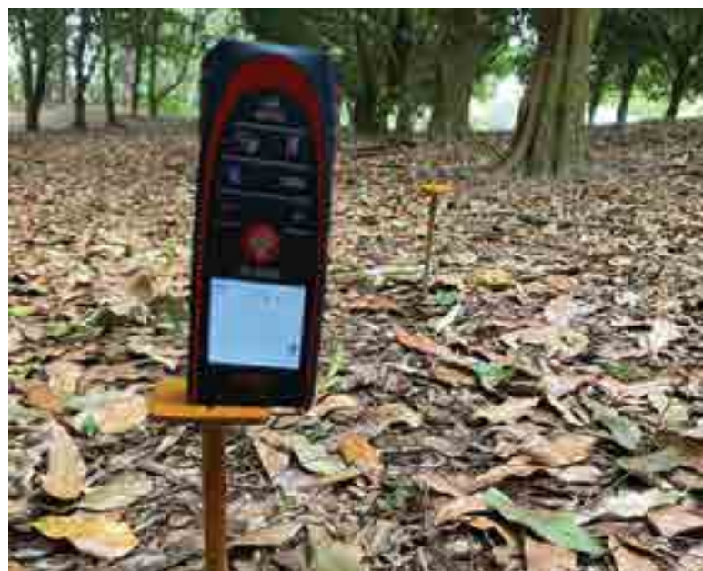
The laser meter is placed on top of a permanent erosion pin to measure soil and mulch movement.
