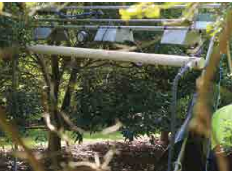
The rainfall simulator's droplet generator heads and pressure gauge.
