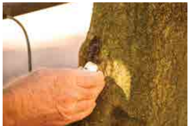
The positioning of sap flow sensors is important to get accurate information. They should be placed in line with the direction of sap flow and in an area that's free from grafts and blemishes.
