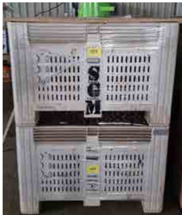
Pallet wrap the sides of the bin and any open sections between the stacked bins and make sure the exhaust fan is extracting air.
