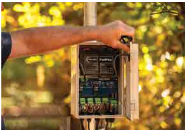
Rimik's data node system takes information from multiple sensors and communicates it to the Farm in One program.
