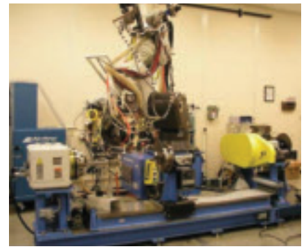
Fig. 2 — Automated laser cell (ALC) for cladding and hardfacing.
