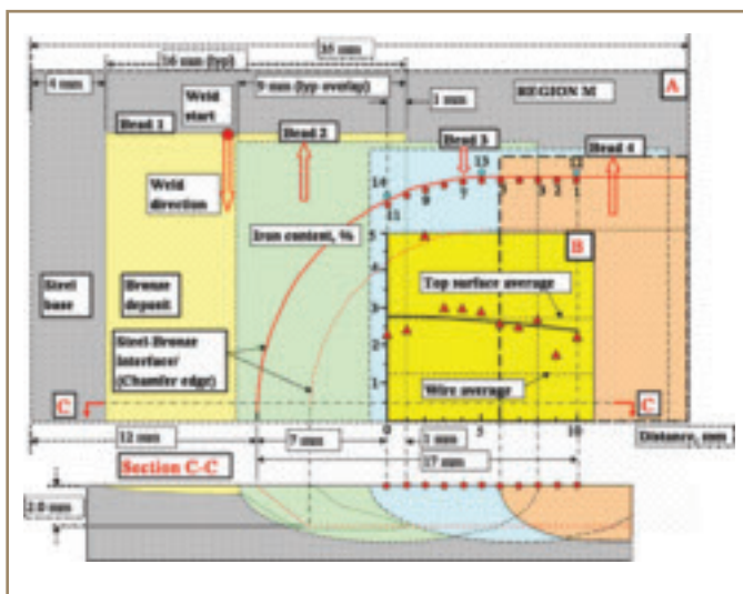
Fig. 7 — A — Schematic of top portion of bearing plate where cladding process begins and shows the directional passes and the corresponding iron (Fe) content along the points; B — results of iron readings superimposed on Fig. 7A.
