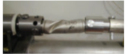
Fig. 11 — Torsion test failure occurs in shaft remote from the weld.
