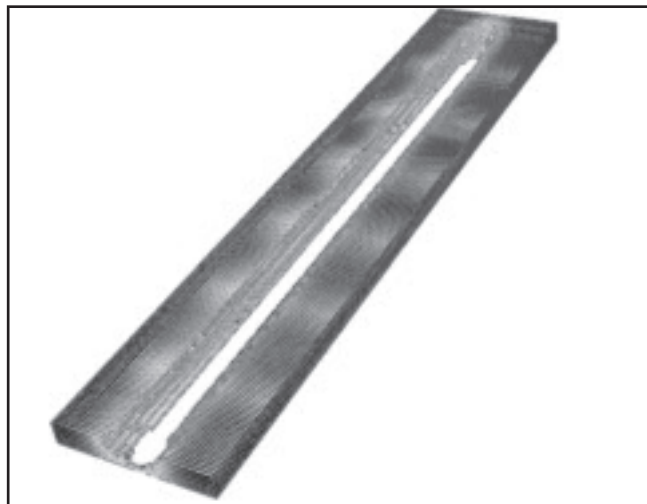
Fig. 6 — Fusion of the workpieces is shown by removing all elements that have been above the melting point. It shows that a complete joint penetration weld is obtained except from the start of welding. At the end of the welding, the weld pool gets wider because the heat input is not able to be conducted away from the fusion zone.
