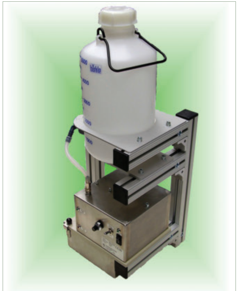
Fig. 3 — Liquid metering pump NB40B886. It is designed to meter between 0.1 and 20 mL/min of neutral aqueous or specified organic liquids with a viscosity of up to 5000 mPa·s. Liquids can be oily lubricants and sliding agents, metalworking fluids, liquid coatings, cleaning liquids, or nonshear stress-sensitive dispersions.
