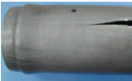
Fig. 12 — Burst test failure occurs in capsule remote from the weld.
