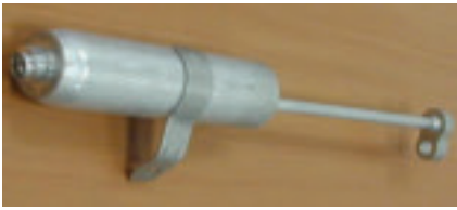
Fig. 6 — Automotive Al A/C receiver dryer.
