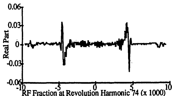
Fig. 5. The linear magnitude of a network analyzer measurement as a function of the DDS RF fraction and time in the acceleration cycle. The RF fraction axis is centered around the 74 revolution harmonic.
