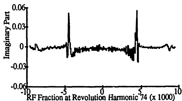
Fig. 7a-c. The magnitude, real, and imaginary response of the network analyzer measurement at a single instant in time centered around 31.5 mS into the acceleration cycle.
