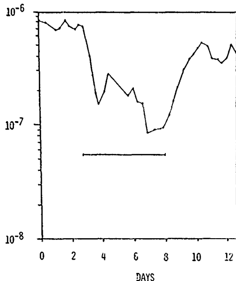
Figure 1. Vacuum scan at A-10 straight section in the AGS ring
