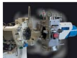
Expansion Control System is an option for the extruder EX1021.
