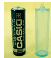
Photo 2 Left: Conventional battery Right: Methanol cartridge (PET bottle)
