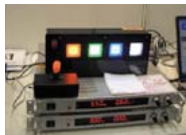
Prototype of a Four-Color Field Emission Lamp Using Thin Nano- diamond Film
