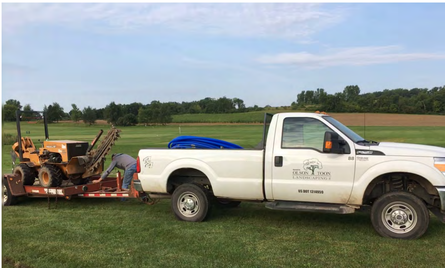
Justin Johnson Olson-Toon Landscape brought out a trencher and wire puller to install irrigation wires.
