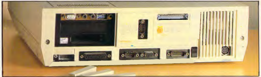
To install one expansion card, six plastic covers must be removed
