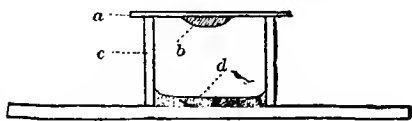
Fig. 66. — Böttcher's Moist Chamber. a, Cover glass; b, droplets of nutrient material; c, glass ring; d, water.
