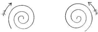
FIG. 5.—Diagram showing section of a vortex ring in its first stage. The arrows indicate the direction of the motion of the molecules (Hovenden).
