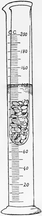
FIG. 174. Device for weighing and determining the volume of seeds.
