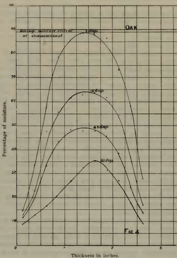
GRAPHS ILLUSTRATING THE PROGRESSIVE DRYING OF 3 IN. TIMBER AT 40°C AND 50% HUMIDITY.
