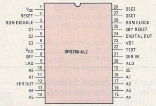
FIG. 1—PINOUT DIAGRAM for the SPO256-AL2. Refer to text for a detailed explanation.
