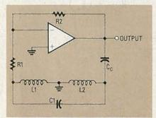
FIG. 6—THE HARTLEY OSCILLATOR is composed of a two-inductor, one-capacitor feedback network.
