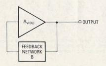
FIG. 1—A FEEDBACK OSCILLATOR may be considered theoretically as an amplifier and a feedback network.
