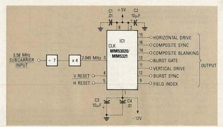
FIG. 9—IF NO DECODING SIGNAL IS AVAILABLE, this circuit can use the 3.58-MHz color-burst signal to reconstruct all of the components of an NTSC sync signal. the circuit should be an amplified version of the video signal, with all traces of the encoding signal removed.
