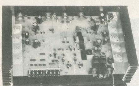
FIG. 10—MOST SWITCHES AND POTENTIOMETERS are soldered directly to the PC board; that eliminates much tedious wiring by hand.
