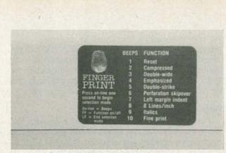
A LABEL AFFIXED TO THE FRONT of the printer tells what functions can be programmed directly from the printer's controls. This label for the IBM Graphics Printer shows 10 beeped functions.
