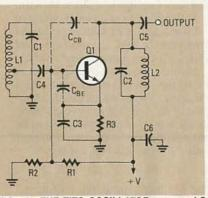
FIG. 10—THE TITO OSCILLATOR uses an LC tank at both the input and output of the circuit; the two tanks are tuned near, but not precisely at, the same frequency.
