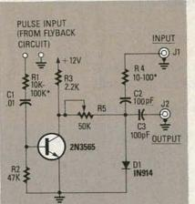
\*DETERMINED EXPERIMENTALLY FIG. 4—THIS SIMPLE DESCRAMBLER is based on a continuously variable attenuator. Though difficult to align, it can be made to work.
