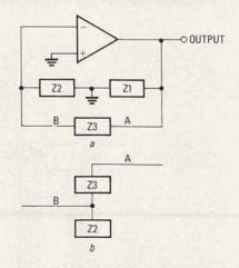
FIG. 2—THE FEEDBACK NETWORK is often composed of three impedances, Z1, Z2, and Z3, as shown at *a*. For purposes of mathematical analysis, Z2 and Z3 may be treated similarly to a resistive voltage divider (*b*).
