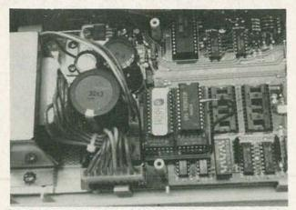
THE PRINTED CIRCUIT ASSEMBLY fits on top of existing hardware. Depending on the printer, the two empty sockets to the right of the Fingerprint might be filled with ROMs: Just ignore them. They don't get in the way because the circuit board sits above them.
