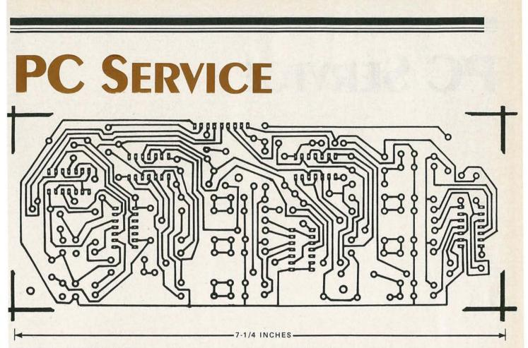
THE CONTROLLER BOARD for the FET power amplifier can be built using this single-sided PC board. The pattern for the main board is shown on page 64.
