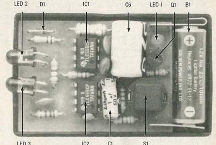
LED 3 IC2 C1 S1 FIG. 5—THE COMPLETED TRANSMITTER appears as shown here. The legs of the electrolytic capacitors (C1 and C6) must be bent horizontally for those capacitors to fit in the case.
