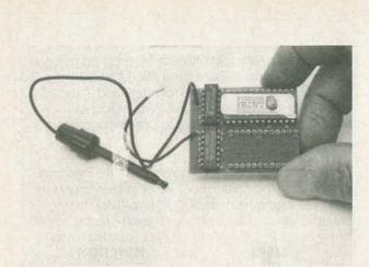
THE IBM GRAPHICS PRINTER and other MX -80 based models need a small printed circuit assembly that substitutes for the existing printer ROM. The parallel rows of terminals on the board create a 24-pin socket to which the original ROM is moved. The mini-clip provides a solder-free connection to exisiting printer wiring.
