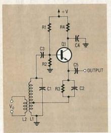
FIG. 8—A HARTLEY OSCILLATOR can also be built using a transistor; oscillating frequency is set by L1 and C1.
