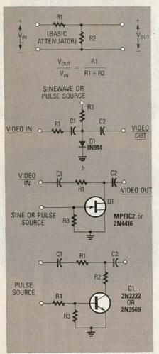
FIG. 3—FOUR ATTENUATOR CIRCUITS. A basic fixed attenuator is shown in *a*. The attenuators shown in *b* and *c* are continuously variable. The attenuator in *d* has an on/off operating characteristic.
