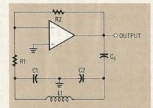
FIG. 5—THE COLPITTS OSCILLATOR is composed of a two-capacitor, one-inductor feedback network.
