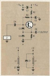
FIG. 7—A COLPITTS OSCILLATOR can be built using a transistor (a). The block marked Z should be replaced by the network shown in b (for a Clapp oscillator) or c (for a pure Colpitts oscillator).
