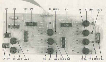
FIG. 12—THE COMPLETE CONTROL BOARD appears as shown here. Capacitors C2 and C3 must be bent flat against the board so that it won't interfere with the front panel.
