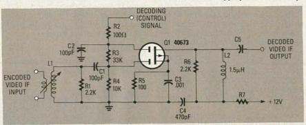
FIG. 6—THIS DESCRAMBLER IS based on a variable-gain amplifier. The decoding signal is used to determine the amount of the gain.
