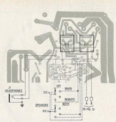
FIG. 14—THE LEFT REAR CORNER OF THE MAIN BOARD is shown here. The headphone jack (J1), the speaker switch (S12), and two jumpers are wired to the row of pads in front of the relays. The wires to J1 are routed above the PC board; the remainder are routed below the board.
