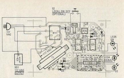
FIG. 6—COMPONENTS MOUNT ON THE RECEIVER BOARD as shown here. One shield must be soldered to each side of the board after testing confirms that the preamplifier works.
