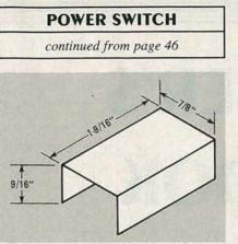
FIG. 7—CUT AND BEND THE UPPER SHIELD from a thin piece of tin as shown here. until you get some response from the circuit. Don't worry about making an exact adjustment. The adjustment we're doing now is preliminary; the receiver must be fine-tuned to obtain maximum range of about 30 feet.
