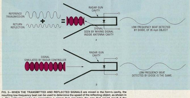
resulting low-frequency beat can be used to determine the speed of the reflecting object, as shown in a. The calibrator works by generating a signal that simulates the one that would result if the transmitted signal were reflected by an object moving at a specified speed, as shown in b. As a result, the low frequency beat detected by the diode is the same as the one in a.
