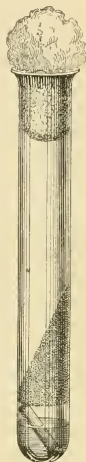
FIG. 209.—Cotton plugged tube with a potato slant resting on a bit of glass rod to keep the potato out of the water in the bottom of the tube. (After Williams, in Schneider, Pharmaceutical Bacteriology , p. 54.)
