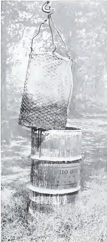
FIGURE 13.—Apparatus for acid treatment of black locust seeds.
