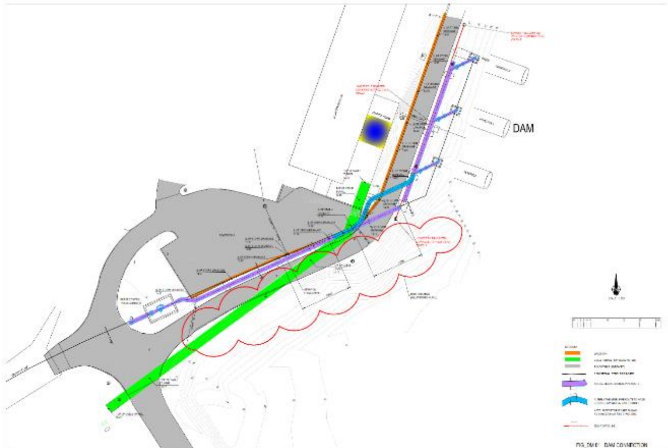
Figure 3-4: Top view of the line routing at the intake structure at Mt Coffee HPP
