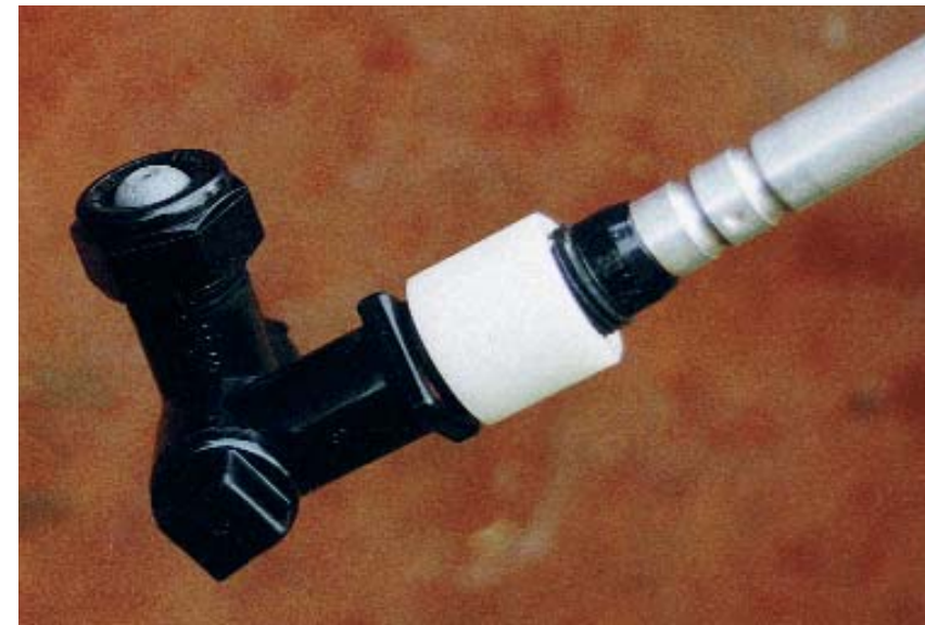
13. V lance with swivel joint to allow the nozzle to point upwards
