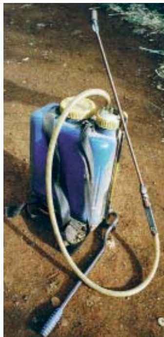
9. Lever-operated knapsack sprayer
