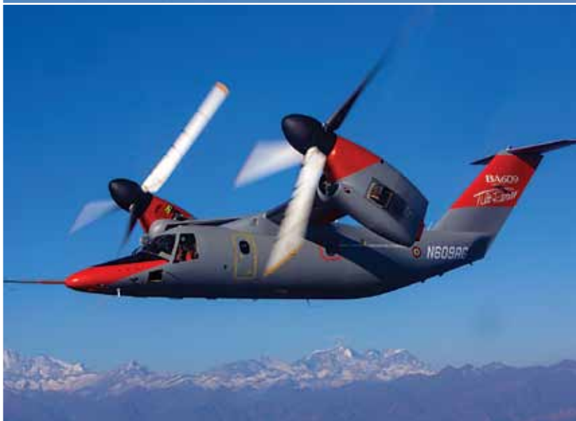
Leonardo introduced modifications (above) to the AW609’s rear fuselage and tail fin in 2013. The original design (below) was the product of extensive wind tunnel testing early in the program.
