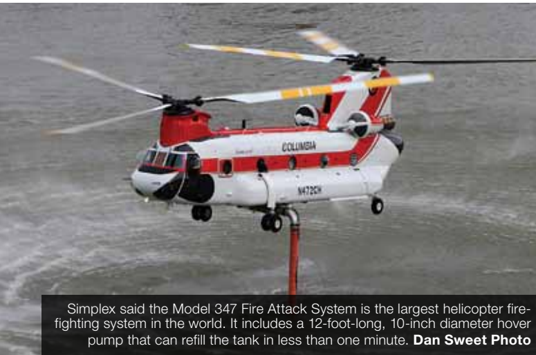
Simplex's belly tanks are made from carbon fiberglass material for durability and low weight. All systems are ground fill and hover fill capable, and can carry foam retardant or water.
