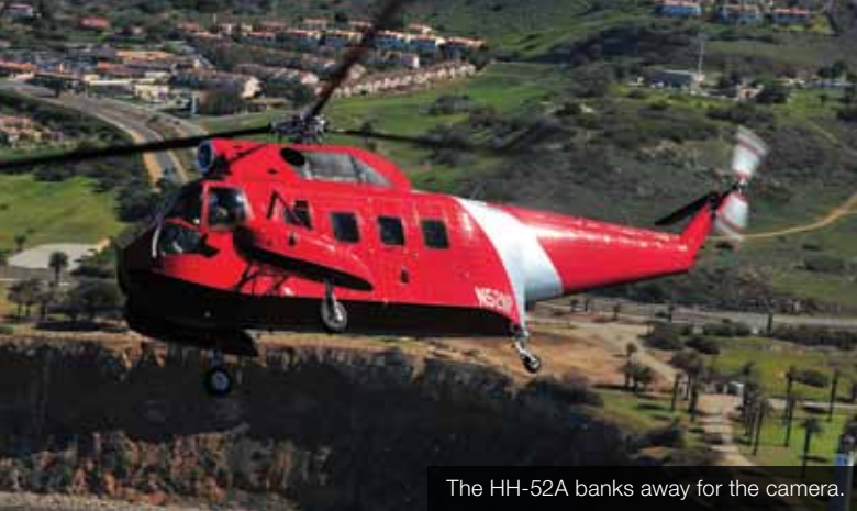
The HH-52 uses the Sikorsky S-55 drivetrain and a single T-58 turbine engine, as used in the SH-3 Sea King.
