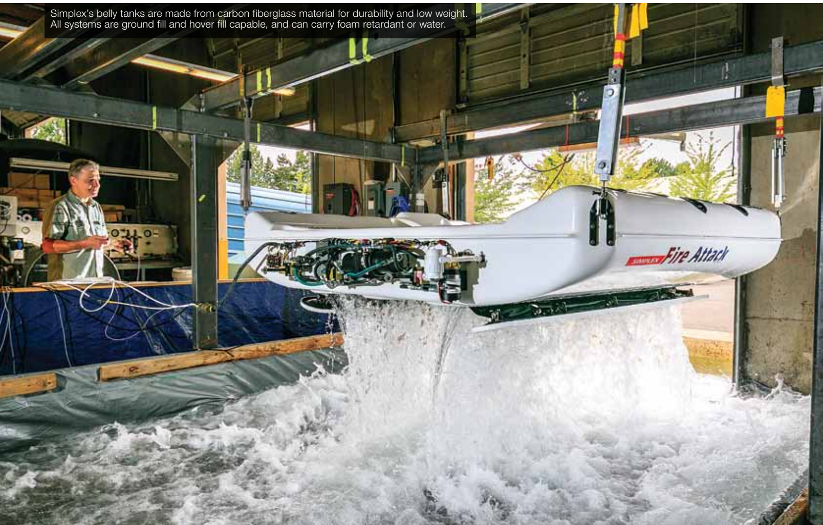
Simplex said the Model 347 Fire Attack System is the largest helicopter fire-fighting system in the world. It includes a 12-foot-long, 10-inch diameter hover pump that can refill the tank in less than one minute. Dan Sweet Photo
