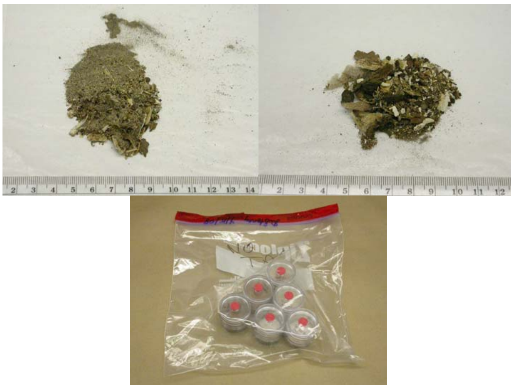
Figure 2. Debris recovered directly from fabric bags (top left), from the bottom of the box (top right) and by using vacuum cassettes (bottom).
