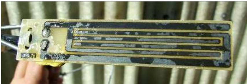
Fig 11.1 Damaged leaf wetness sensor.
