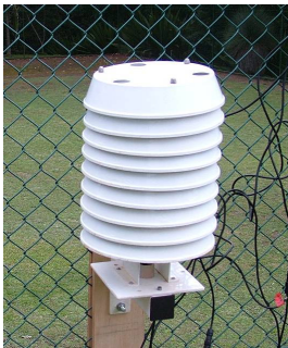
Fig 11.7 Stevenson screen containing temperature and RH sensor.
