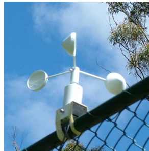
Fig 11.8 Wind speed anemometer.
