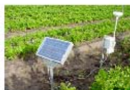
Weather station used to collect temperature and leaf wetness information
