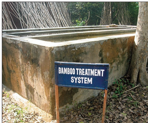
Fig. 1: Tank for dipping of bamboo samples
