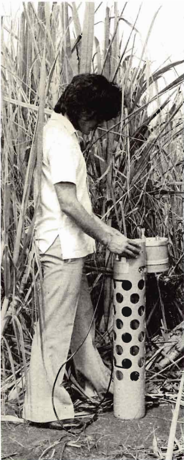
Plate II. The Wallingford Neutron Probe for soil moisture determination and (right) close-up of its rate scaler.
