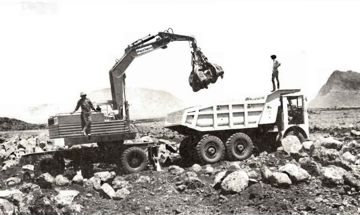
Plate VII. Boulders encountered in cane fields and their removal after being shattered.
