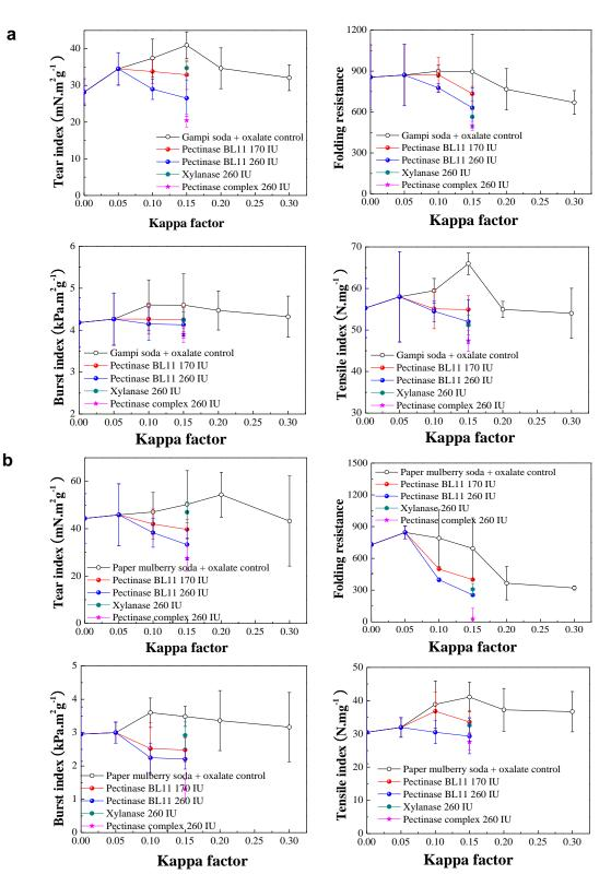
**Fig. 4.** Effect of enzymes on handsheet properties of (a) gampi soda pulp with oxalate and (b) paper mulberry soda pulp with oxalate. Data provided as the mean of triplicate  $\pm$  the standard deviation.
