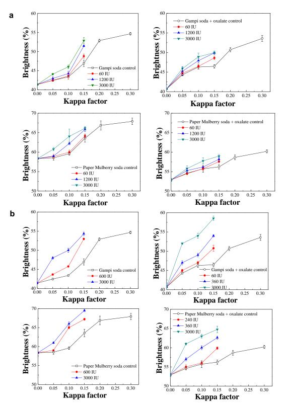
**Fig. 1.** Impact of different dosages of (a) xylanase and (b) pectinase on the brightness of pulp. Data provided as the mean of triplicate  $\pm$  the standard deviation
