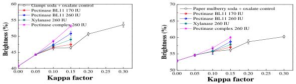
**Fig. 2.** Effect of enzymes on the brightness of pulp. Data provided as the mean of triplicate  $\pm$  the standard deviation
