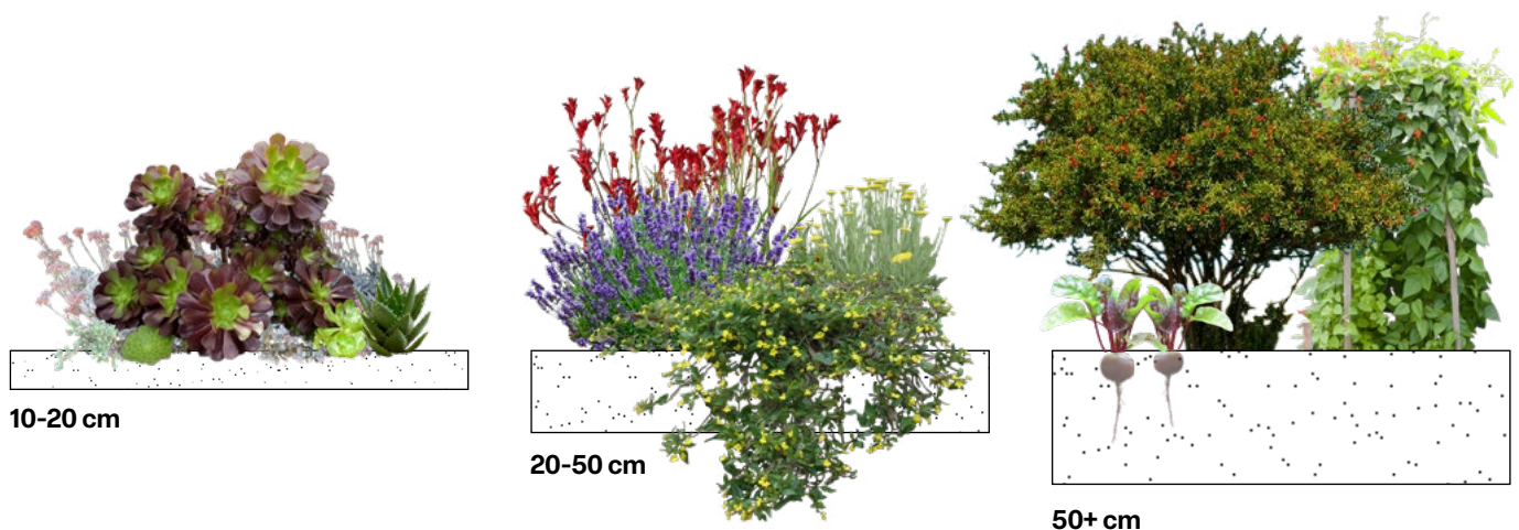
Figure 2.1 Increasing substrate depth increases rooting volume and water storage, supporting larger plants and more diverse plantings.
