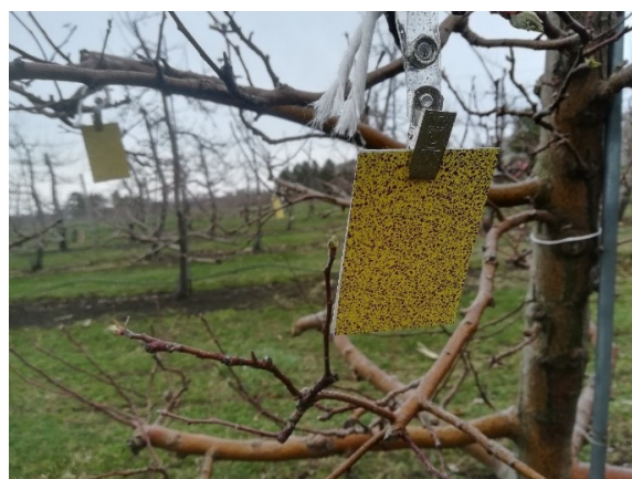
Figure 1. Spray coverage is the percentage of the crop surface on which spray droplets land. Water sensitive paper can be used to visualize coverage.
