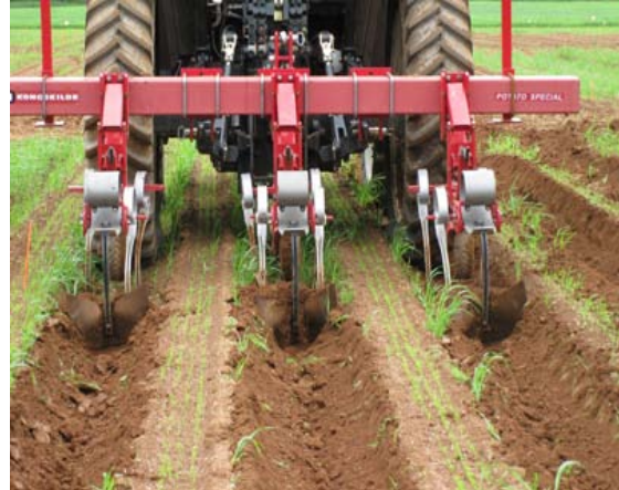
S-tines with shovels for weed control between the raised beds
