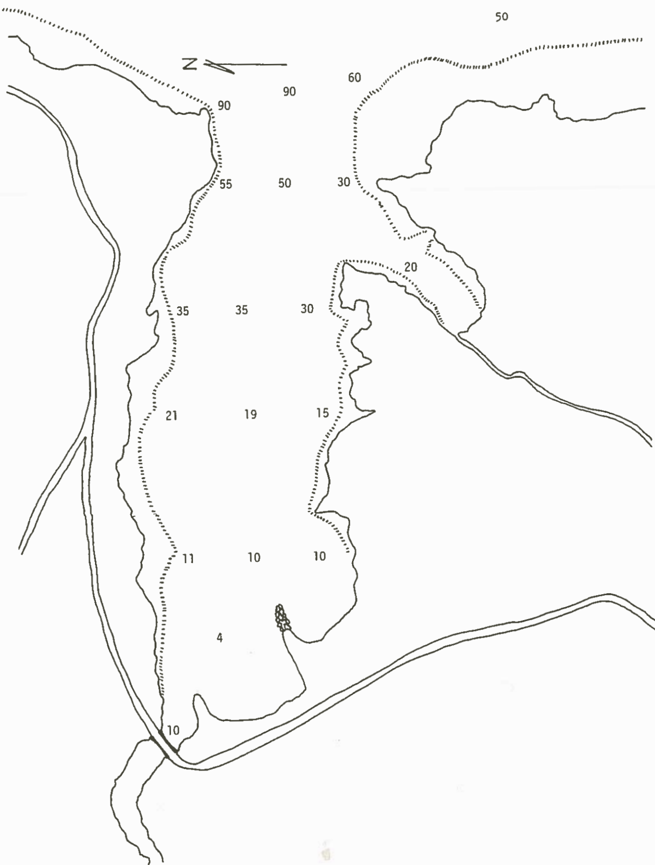
Figure 37. Locality map for soundings taken in Talofofu Bay. Depths are given in feet.
