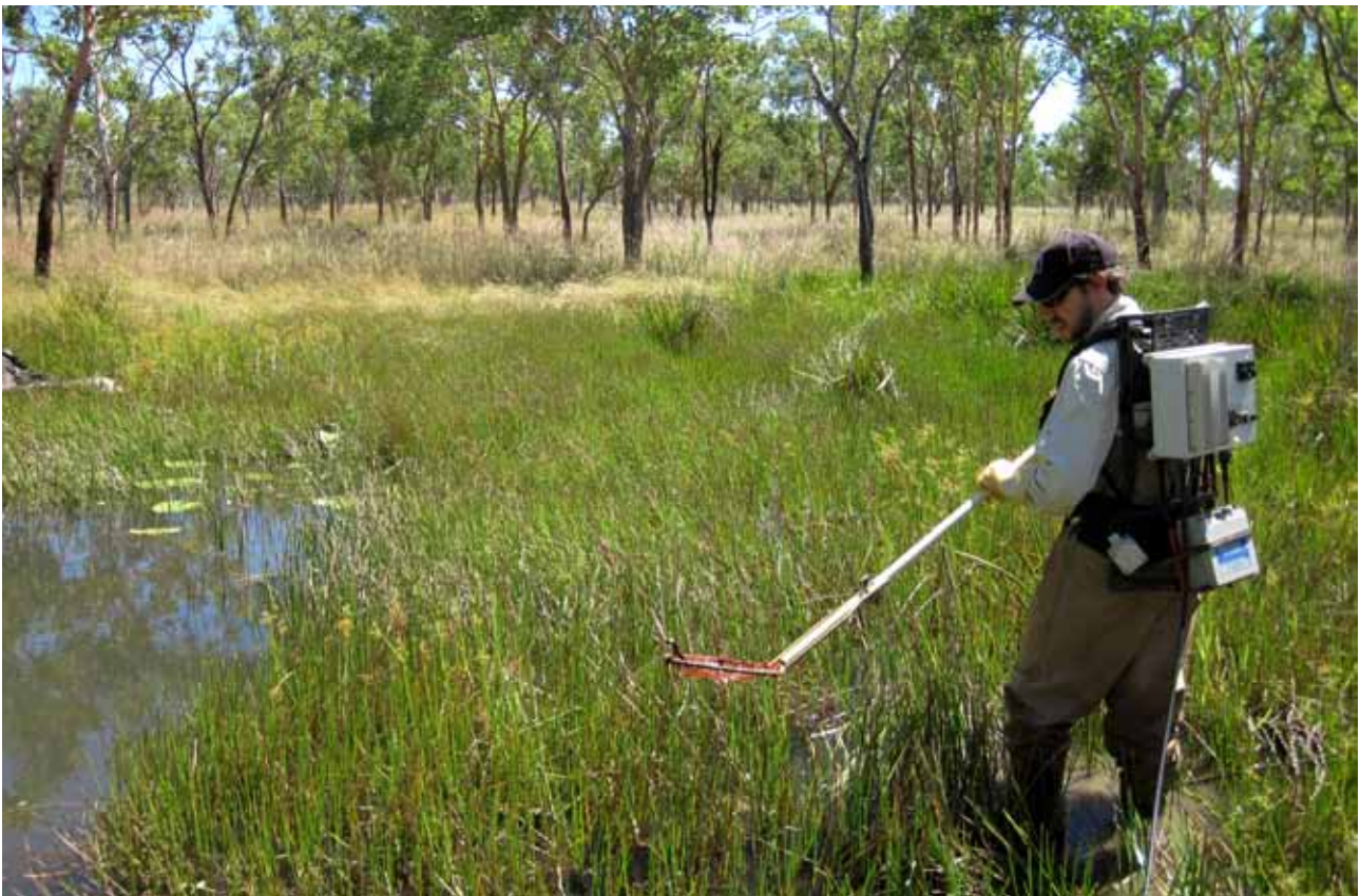
Electrofishing uses electricity to stun fish so they can be easily surveyed. The fish return to their natural state unharmed, shortly after being stunned © Copyright, D. Wilson
