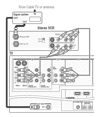
**Note:** The VIDEO/AUDIO OUT terminals output signals from the ANT 1, ANT 2, VIDEO 1, VIDEO 2, and VIDEO 3 terminals when the appropriate input mode is selected.
