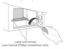
**NOTE:** Make sure the lamp unit and screws are installed securely; otherwise, the TV may not turn on and the lamp life may be shortened.
