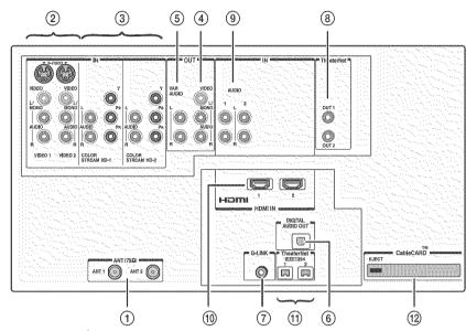
① ANT-1 (CABLE) IN and ANT-2 IN — Two inputs that support analog (NTSC) and digital (ATSC) off-air antenna signals and analog and digital (QAM) Cable TV signals.
