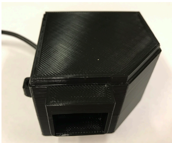
The Texas Instruments DLP NIRscan Nano EVM. The miniature NIR scanner can be powered by a USB connection or by battery. The device comes without a case, so Cam-core is developing cases that can be produced with a 3D printer.
