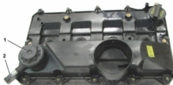
2 – Tappet cover oil vapour recovery pipe
