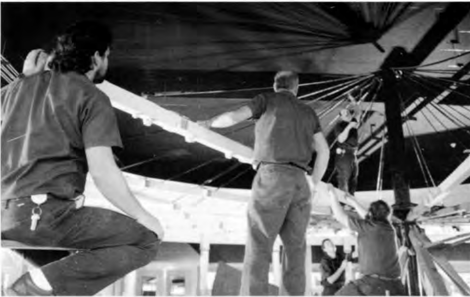
Piece by piece the carousel is dismantled. Here the sweeps are removed. The old mechanism was unreliable and the Children's Museum felt new equipment would run better.
