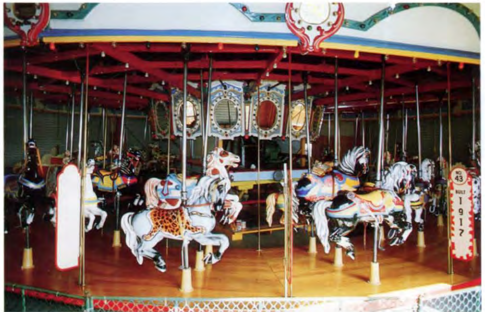
PTC 43 was built in 1917, one of only three portables listed in the company's records. The centerpole is mounted on a wagon. Forty-two jumpers, two chariots and two standers ride the platform.
