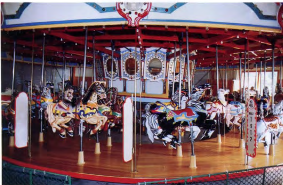
Note the armored jumper on the left of this photo, and compare it to the photograph on the adjoining page. Also note the hinged panels. They dissuaded patrons from getting too close, and helped prevent riders from jumping on without a ticket.
