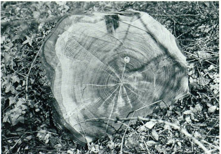
Plate 6: Star shake in oak (p. 59). The splits are stained and run deep into the log. G. S. Henman
