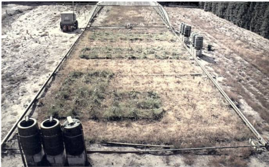
Plate 5.1 Rothamsted mobile rain shelter used in experiments to simulate drought conditions (Expts 4 and 5).
