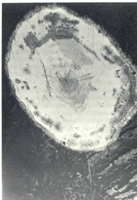
Plate 19.2 Watermark stain in the cut bole of a cricket bat willow.
