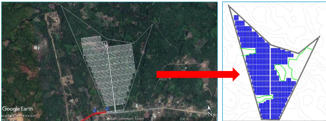
Figure 12: Site layout alternatives showing the original layout with the revised based on site sensitivities
