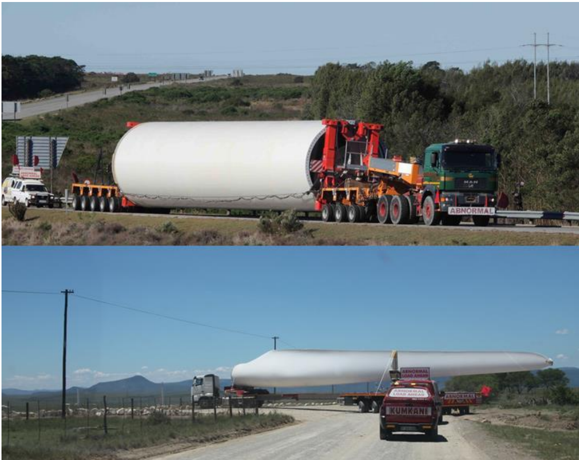
Figure 2-16: Tower section in low load configuration shown in top figure and blade shown in bottom figure
