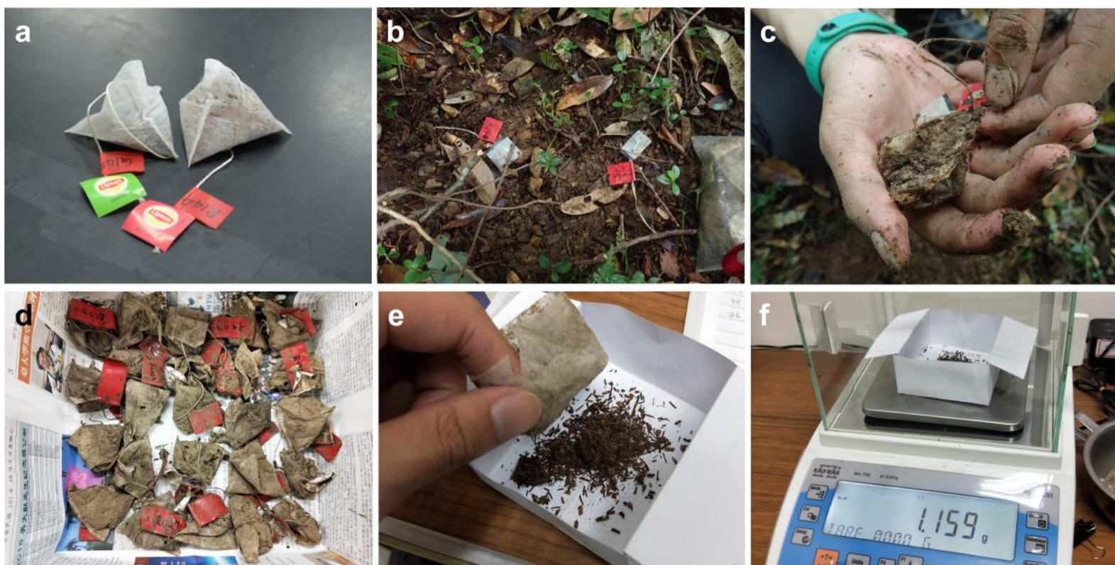
Figure 1. (a) New teabags prepared for the experiment. (b) Teabags buried in the soil, with tags visible on the surface. (c) After ca 90 days, teabags were dug out. (d) After drying 48 hours at 70°C, teabags were ready for weighting. (e) Each teabag was opened and the tea remnants weighted. (f) Measuring the weight of decomposed tea. The process of teabag excavation in Taiwanese lowland sub-tropical forest can be also seen on this video: https://vimeo.com/390990611/3ca00eca4f .
