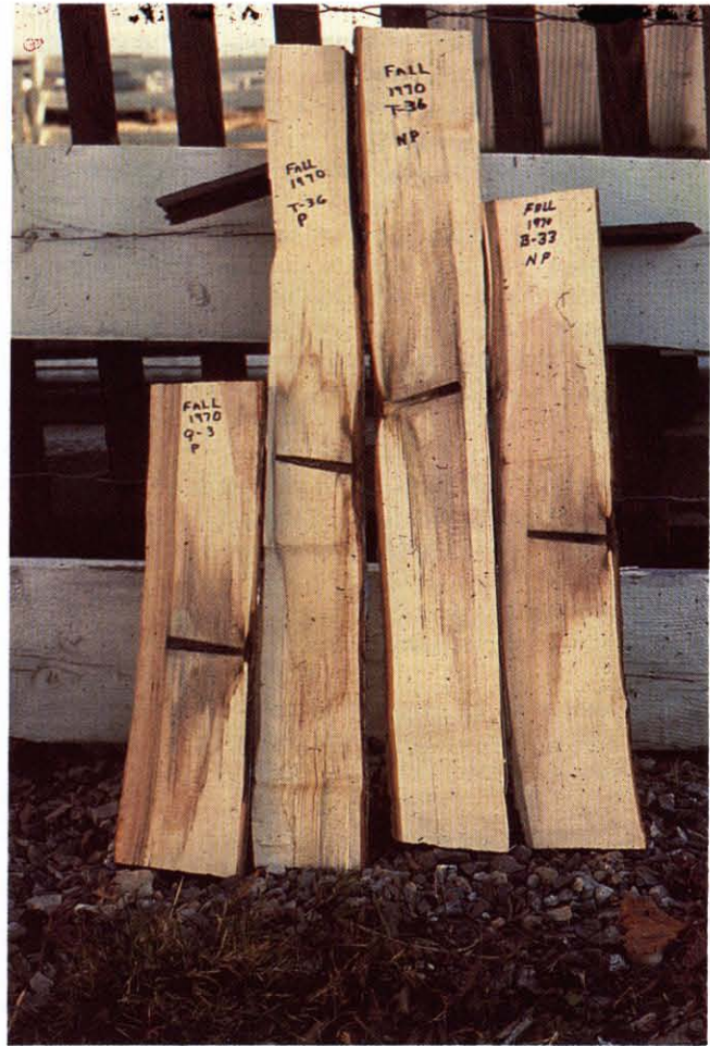
Figure 6.—In radial section, discoloration in the wood extends for some distance above and below the taphole. Tapholes in sections marked “P” had been treated with paraformaldehyde.
