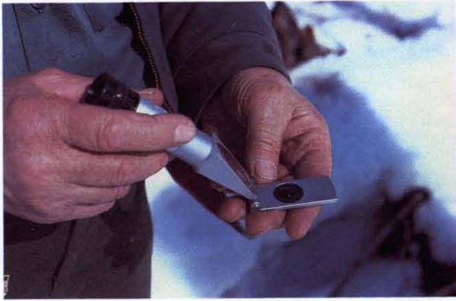
Figure 3.—A sugar refractometer, used for measuring sap sweetness, in the open position.
