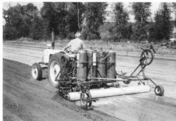
Figure 1. Continuous tarp fumigation consists of glued, overlapping sheets of fumigation tarp which form a solid cover.
